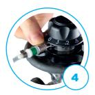
Secure the connection with the tube clamp
