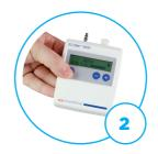
Switch the conserver on by pressing the on/ off button once
