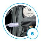
Connect the nasal prongs tubing to the connection on the side of the conserver
