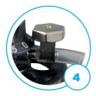
Secure the connection with the tube clamp
