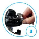
Connect the coiled tubing to the outlet connector on the cylinder
