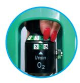
Check the cylinder is switched on properly and set to the correct flow rate
