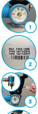
Check the contents gauge to see how much oxygen remains. If the gauge is showing red, your cylinder is empty and needs to be changed immediately.
