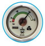
Check the contents gauge to ensure the cylinder is not empty
