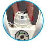
Check the cylinder is switched on properly and set to the correct flow rate
